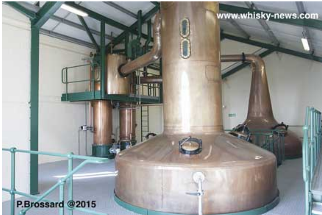
The new type of Lomond's still, as here at Scapa distillery
