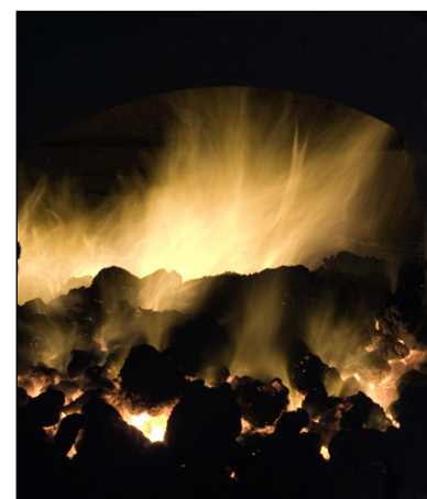
A peat fire inside a kiln to dry the barley and to give a smoky flavour to the spirit.
